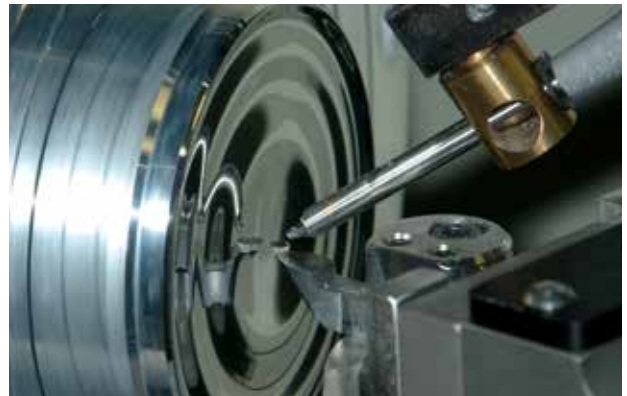
Rotation-symmetric multiple aspherical surface, aluminium.
